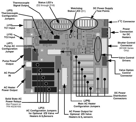
Figure 1-1: Relay PCA Layout (P/N04523)
